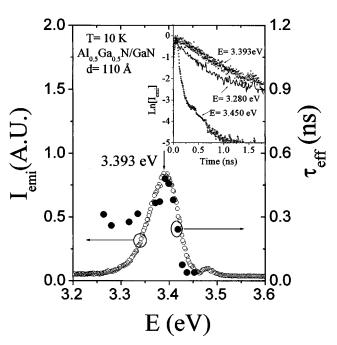
FIG. 5. Emission energy dependence of the decay lifetime of the 2DEG emission line measured at 10 K. The time-integrated emission spectrum is also shown. The inset shows the temporal responses of the PL emission measured at several different emission energies.
