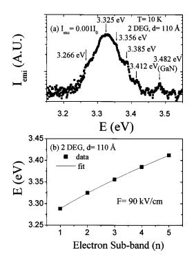
FIG. 4. (a) Low-temperature (10 K) PL spectrum of an  $Al_{0.5}Ga_{0.5}N/GaN$  heterostructure under low excitation intensity (10 W/cm<sup>2</sup>) and five emission peaks are resolved. (b) The least squares fit (solid line) of the observed five emission peak positions (solid squares) with Eq. (1).
