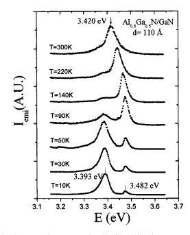
FIG. 2. PL spectra of a representative  $Al_{0.5}Ga_{0.5}N/GaN$  heterostructure with d = 110 Å (KSU A-166) measured from 10 to 300 K.
